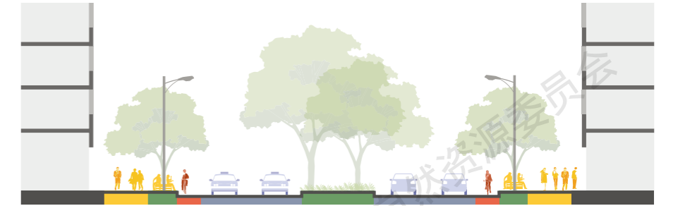
中央式情形之二：机动车道数较多时，在中央林荫道设置林荫景观带 Case 2: When there is a large number of motor vehicles, a tree-lined landscape belt is set up along the central avenue
