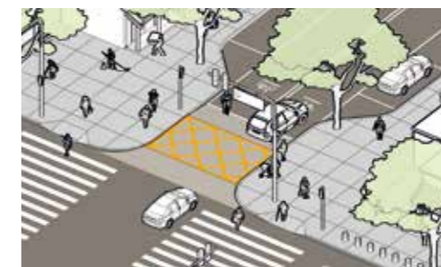
抬升式交叉口人行过街横道示意图 Lifted intersection pedestrian crossing street
