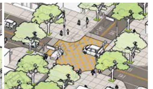
整体抬升式交叉口 Overall raised intersection
