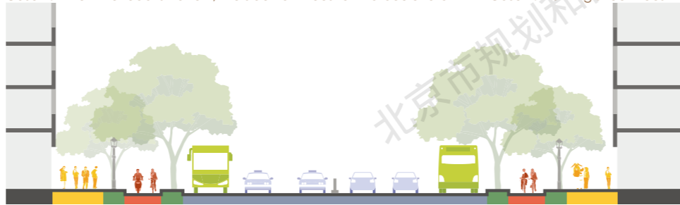
对称式情形之三：道路较宽时，非机动车道两侧各种植一行行道树形成林荫道 Case 3: When the road is wide, trees are planted on both sides of the non-motor lane to form a boulevard
