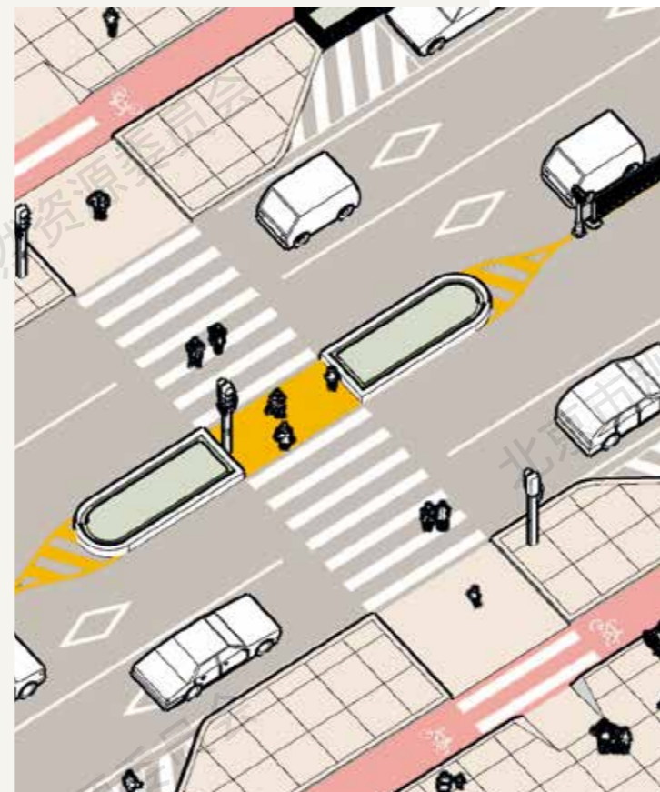
通过车道收窄形成安全岛 To form a safe island by narrowing the lane width
