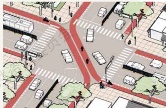
非机动车道左转道设置及标识 Left turn lane setting and identification of non-motorized lane
