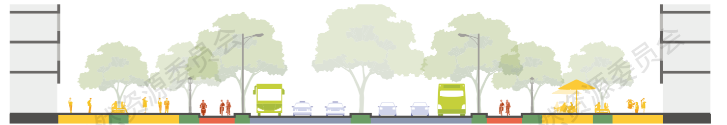
对称式情形之二：在绿化带、设施带、机非隔离带、中央隔离带等的三处以上均种植行道树，形成多个林荫道 Case 2: Planting street trees in more than three places such as green belts, facility belts, non-isolated belts, and central isolation belts, to form several avenues
