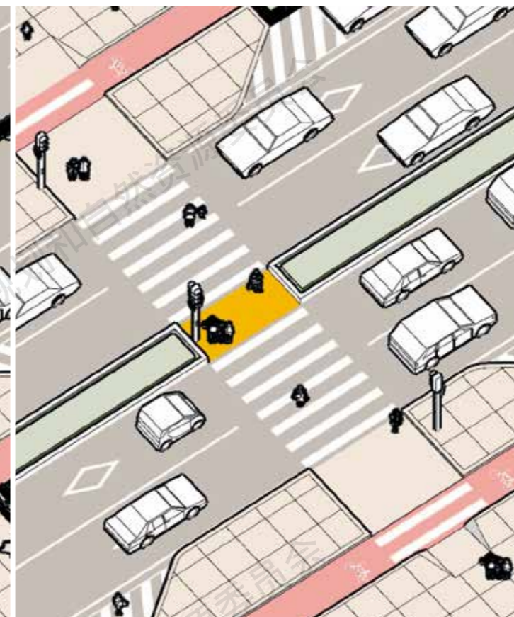
利用中央分隔带设置安全岛 To set up a safe island with a central divider
