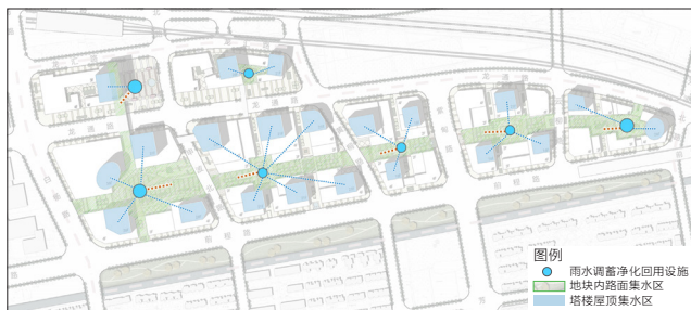
图6 塔楼雨水收集回用系统示意图 Fig.6 Rainwater collection and recycling system of tower
