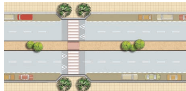
Figure 5.18 Curb Extensions Create Parking Pockets
