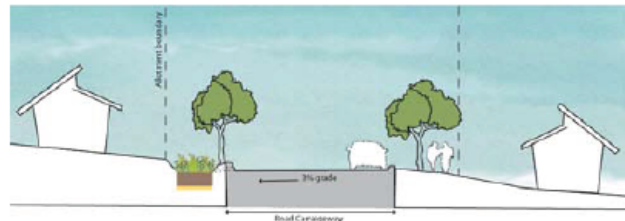
Figure 23 — WSUD street layout 2: Streets aligned parallel (or tangential) to the contour with allotments on both sides of street
