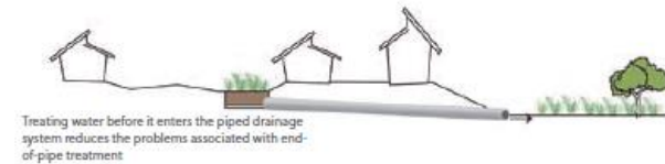
Figure 17 — Benefits of treating stormwater at-surface on flat sites (Hoban, Eadie and Rowlands, 2007)
