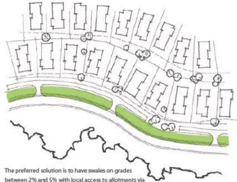
On steep and undulating sites, roads should be aligned to reduce the grade. The suitability of swales on moderate slopes (2% to 5%) is increased, but the presence of driveway crossovers can be problematic.
