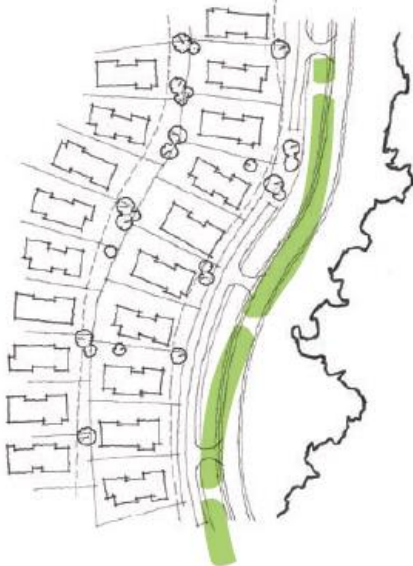
Figure 20— Shared driveways can achieve separation between allotments and swales
