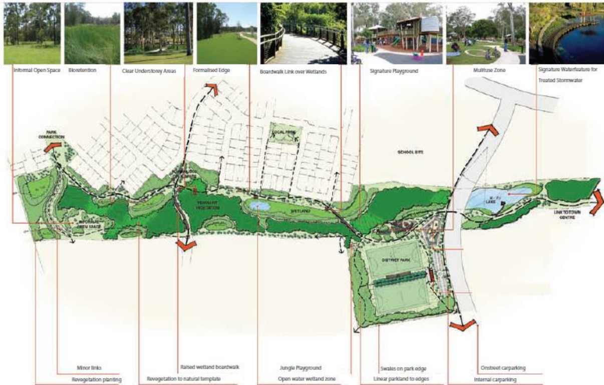
Figure 21 — Multiple use open space corridor incorporating WSUD BMPs, a constructed wetland and bioretention systems to treat stormwater runoff from adjoining development areas.
